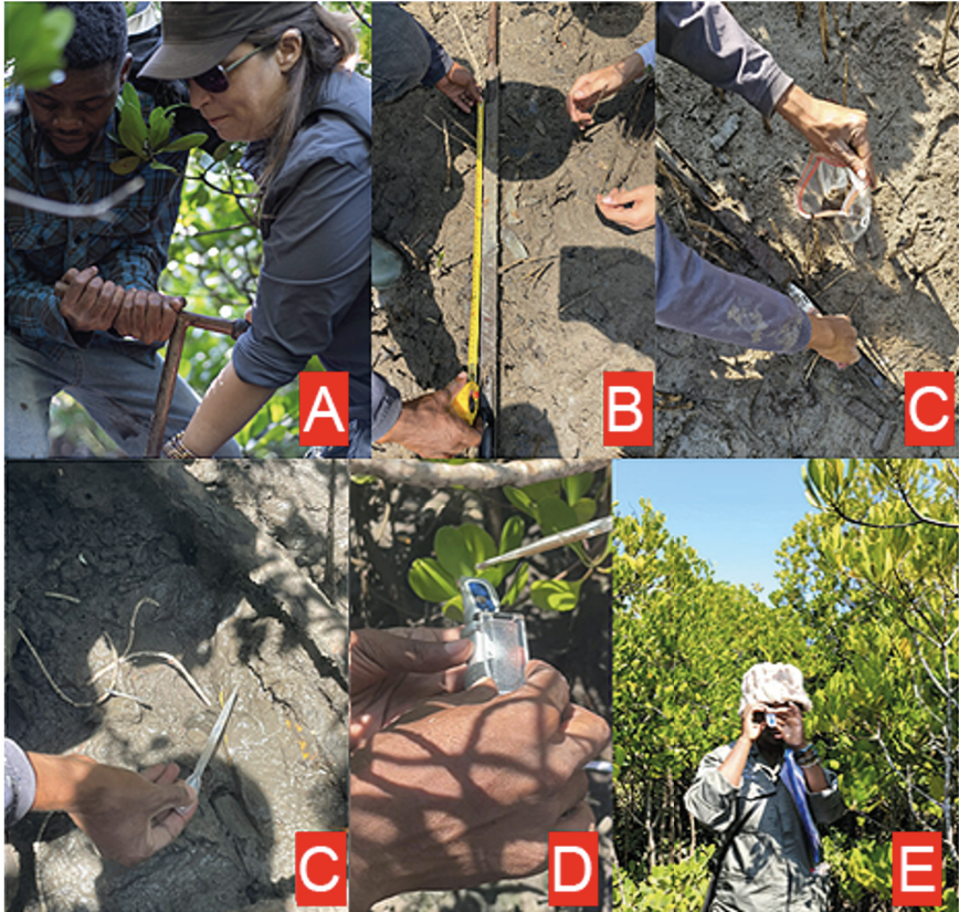
Figure 3. Sampling moments during fieldwork at the mangroves of Saco da Inhaca. (A) Soil extraction; (B) measurement of soil core length; (C) collection of soil core sections in plastic bags; (D) water sampling using a pipette; (E, F) salinity analysis with a salinometer.
