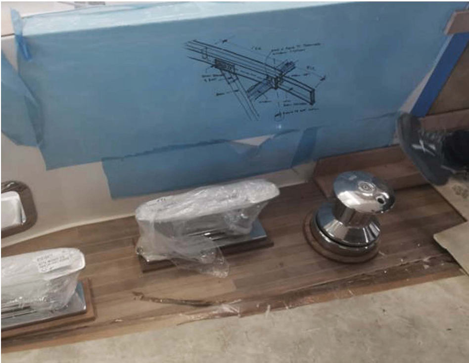
Figure 4. Detail sketch made in production following exchange of ideas between designer and carpenter, Sanlorenzo shipyard, Yacht SL120A.
