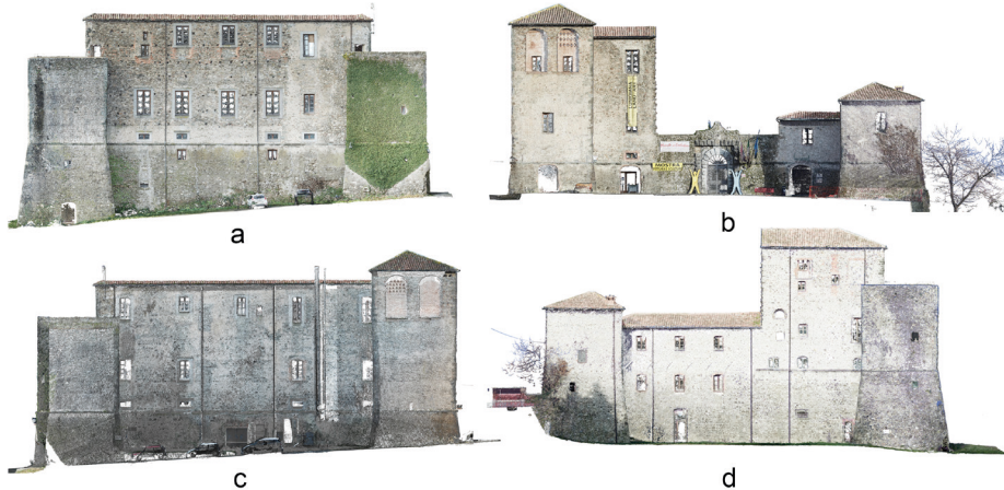
Figure 6. Representation of orthoimages extracted from the aerophotogrammetric point cloud: a. East elevation; b. West elevation; c. north elevation; d. south elevation. (Author's elaboration).
