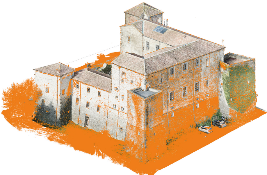
Figure 5. Overlay of the laser scanner point cloud colored in orange with the aerial photogrammetric one to verify the overall accuracy of the project.(Author's elaboration).
