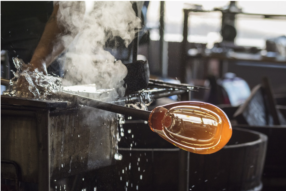
Figure 2. borosilicate glass blowing in the laboratory.
