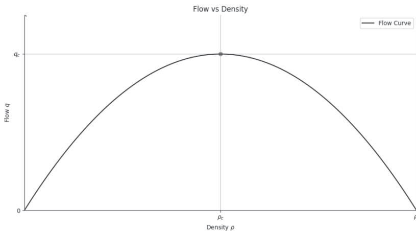
Fig. 4 - Density-flow plot of Greenberg's fundamental diagram
