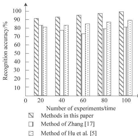
Fig. 2 - Comparison results of obstacle recognition accuracy of three methods in vehicle side blind area
