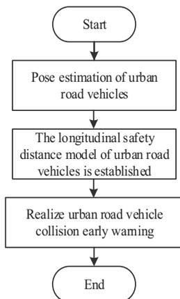
Fig. 1 - Flow chart of vehicle collision warning on urban road
